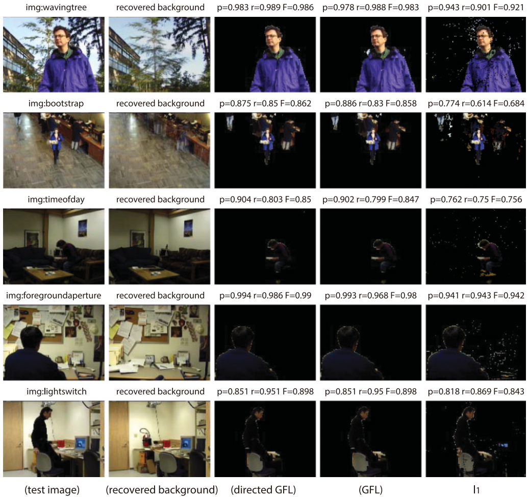
Fig. 9. BS results on the Wallflower dataset. From left to right: Test image, recovered background by directed GFL, BS by directed GFL, GFL, and l_1 .
