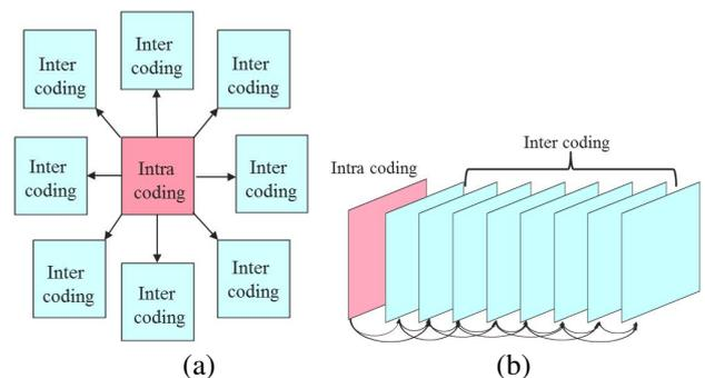
Fig. 1. Prediction structure for image set compression. (a) star topological prediction structure, (b) sequential prediction structure.
