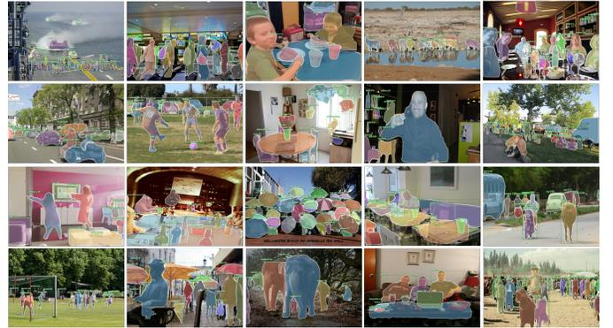
Fig. 3. Example of instance segmentation and detection results on Microsoft COCO 2014, using 512 output feature maps in R-CNN subnet and running at 10 fps, with 28.28 mask AP and 31.85 bounding box AP.
