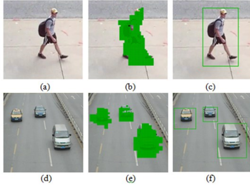
Fig. 8: (a) video data for a walking man with slight shadow; (b) foreground segmentation of (a); (c) bounding box of the walking man in (a); (d) video data in a speedway; (e) foreground segmentation of (a); (f) bounding box of the moving vehicles in (c).
