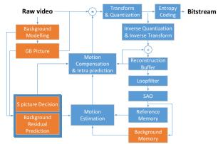
Fig. 1. The architecture of AVS2 scene video coding
